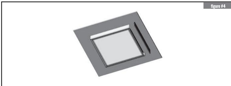
4. Push up luminaire the frame seamlessly.
