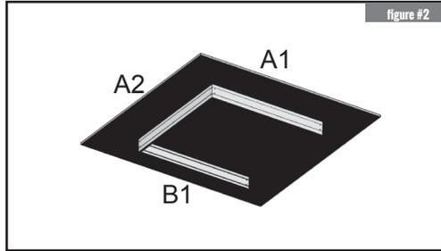
2. Fix the frame to ceiling with screws. Remove the B2 side of the Frame for luminaire installation.
