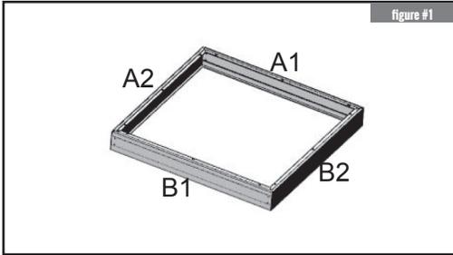
1. Fix A1/A2/B1/B2 with snap-in plastic comers making it a complete frame.
