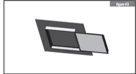
3. Slide partially the luminaire into the mounting frame, as shown. With power turned off at the breaker, connect power to drive based on the wiring diagram.
